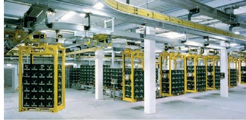
SingleFlexLine 0811 on an electrified monorail system in a brewery
