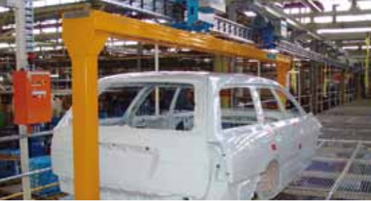
Electrified monorail system with IPT®-Rail and iDAT
