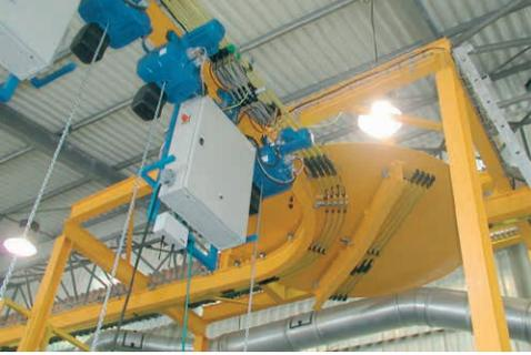
SinglePowerLine 0812 in a galvanizing plant with bridge elements on a turning gate and dual collector assemblies
