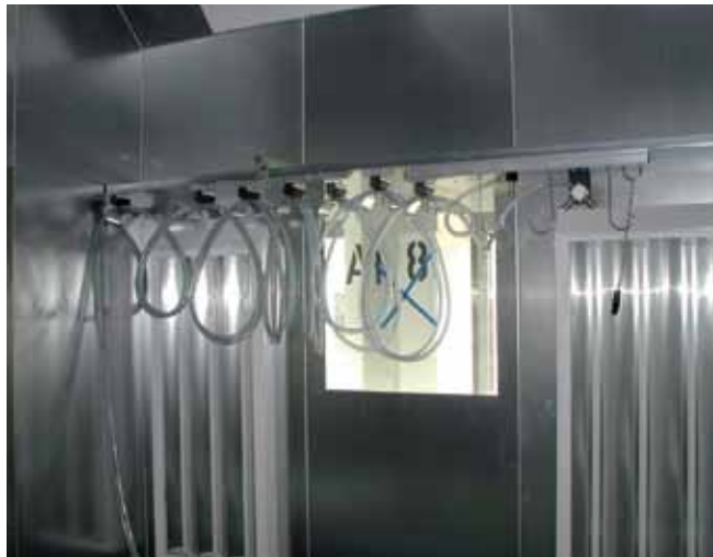
C-Rail system at the finishing area a car production
