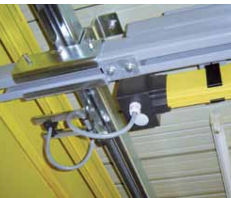
Combined reliability with enclosed conductor rail to an equipment crane .
